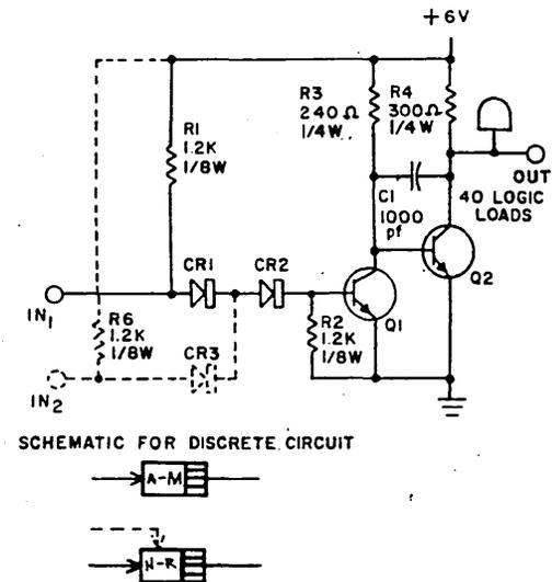
SCHEMATIC FOR DISCRETE CIRCUIT
