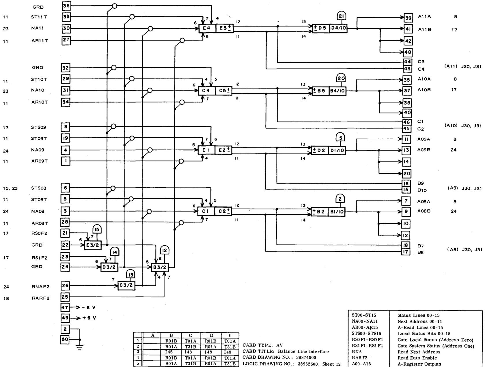
FIGURE 3.18. A-REGISTER INTERFACE: BITS 8-11 (CARD 12)
