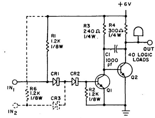
SCHEMATIC FOR DISCRETE CIRCUIT
