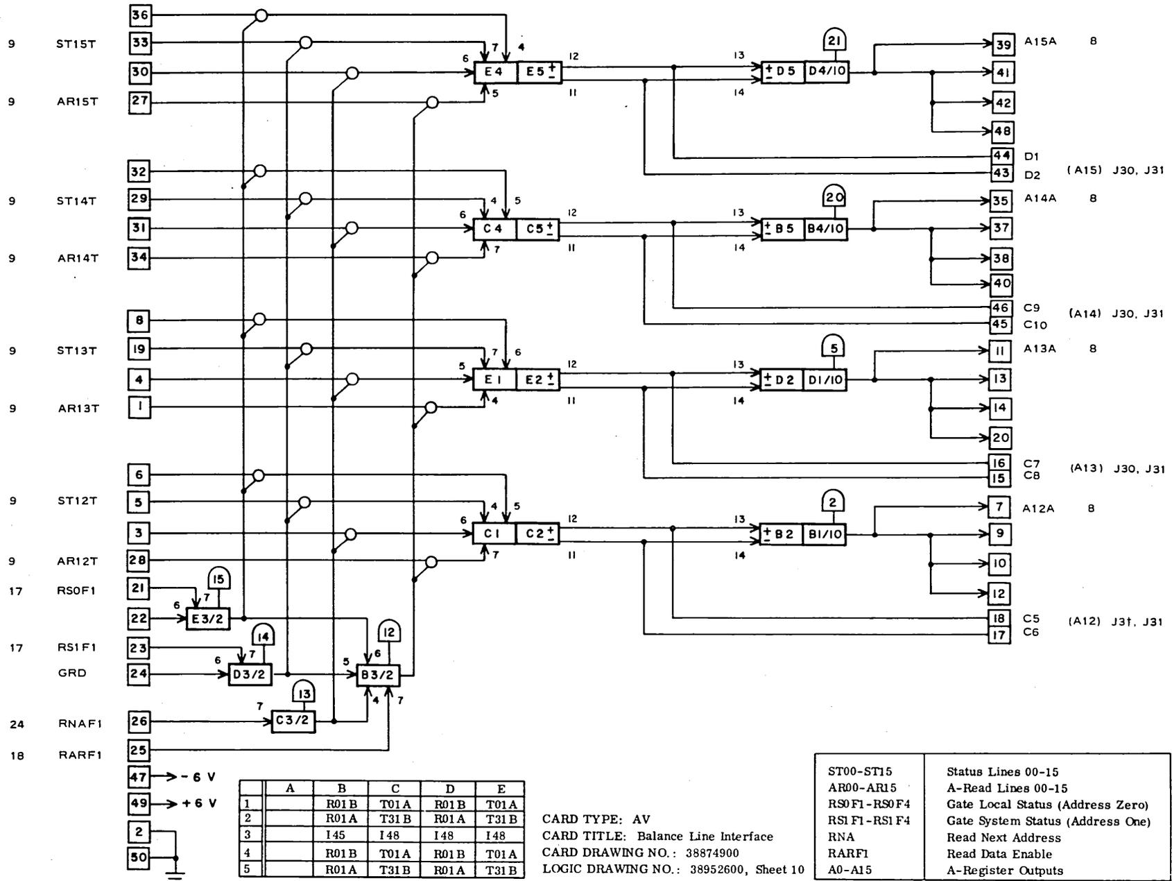
FIGURE 3.17. A-REGISTER INTERFACE: BITS 12-15 (CARD 10)
