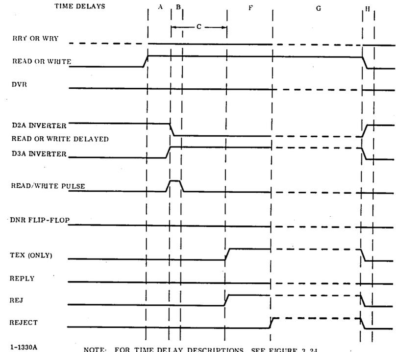
FIGURE 3.27. DEVICE HERE BUT NOT READY CYCLE
