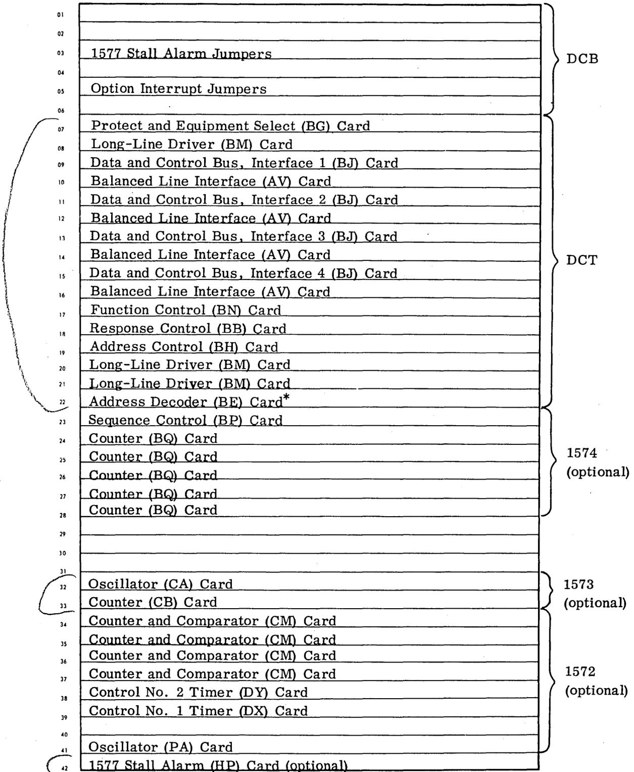
\* Remove Card 22 before installing a 1574 unit.
