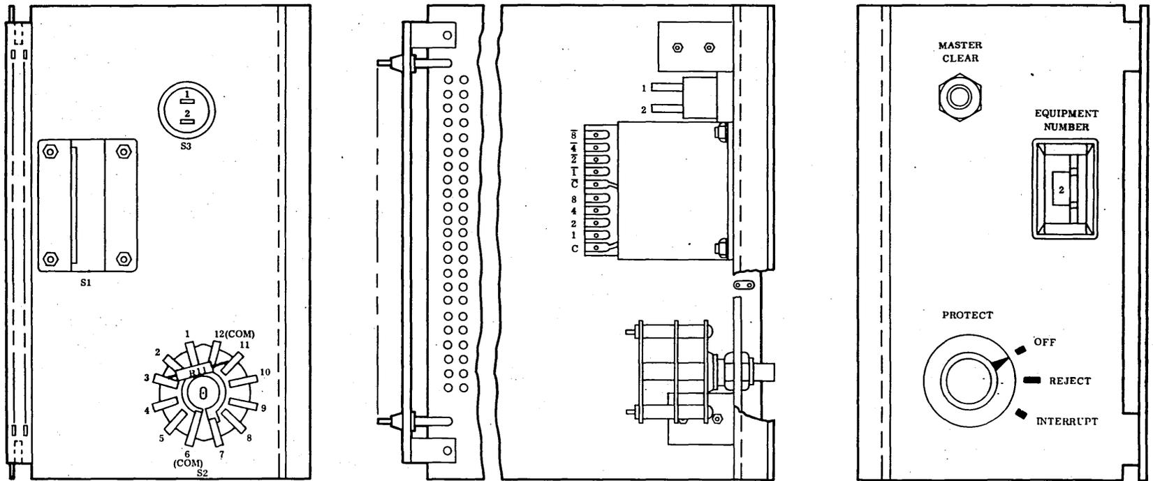
FIGURE 5.4. PROTECT AND EQUIPMENT SELECT (BG) CARD, PANEL ASSEMBLY
