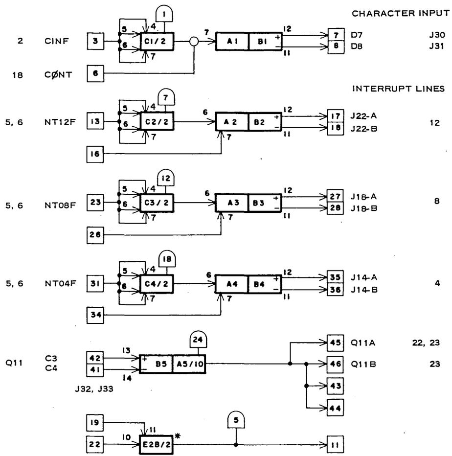
\* NOTE: INVERTER WITH FOUR OUTPUT DIODES TIED TOGETHER
