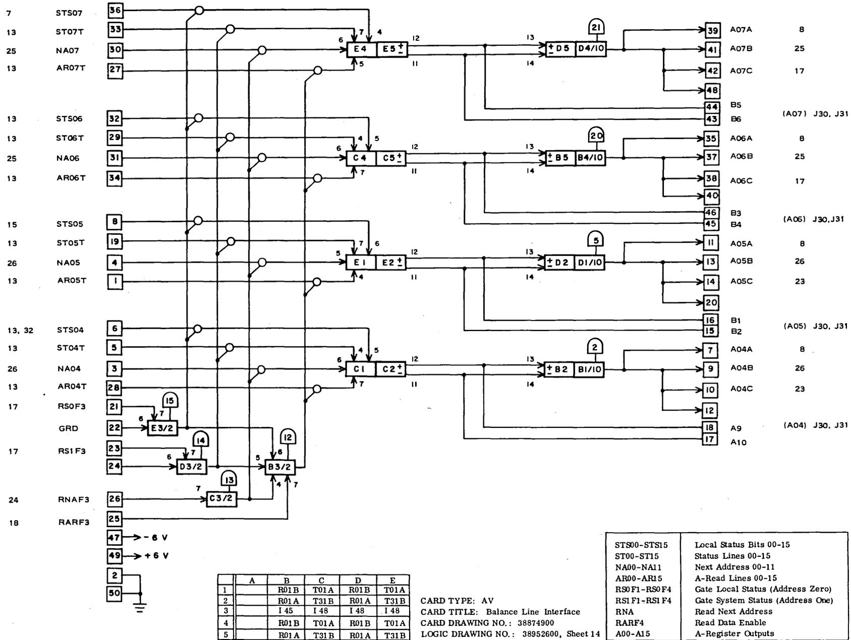
FIGURE 3.19. A-REGISTER INTERFACE: BITS 4-7 (CARD 14)
